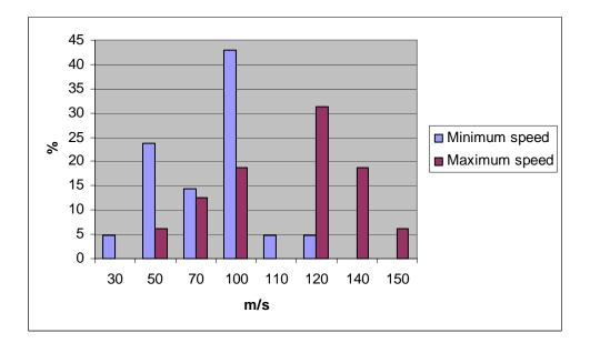
The survey reveals that it would be necessary to look for an aircraft capable of flying at a low speed. Almost half of the participants need a minimum speed of 100 m/s, and over 25% would need around 50 m/s. Mainly, the scientific users interested need low speed for instrument development and for remote sensing campaigns. This is not a difficult requirement to fulfill, as all the aircraft selected in COPAL project (previously identified A400M, C130, C295) could do it.
